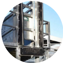
SWIVEL BUFFER BOARD PROTECTS THE RAMP FRAME
