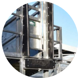
SWIVEL BUFFER BOARD PROTECTS THE RAMP FRAME
