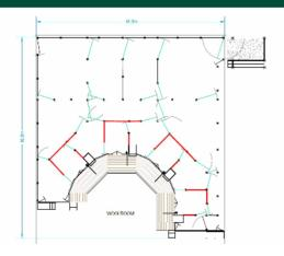
Minimum Shed for Fitout: 24.0mL x 18.0mW x 4.0mH
