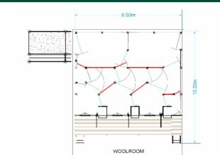
Minimum Shed for Fitout: 18.0mL x 9.0mW x 4.0mH
