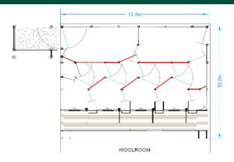
Minimum Shed for Fitout: 24.0mL x 12.0mW x 4.0mH
