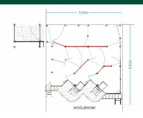
Minimum Shed for Fitout: 18.0mL x 9.0mW x 4.0mH
