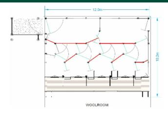
Minimum Shed for Fitout: 24.0mL x 12.0mW x 4.0mH
