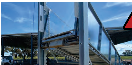
Drop over flap stowed when lifting
